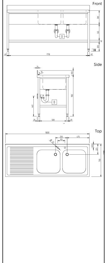
PLUS - Static Preparation 1800 mm Sink Unit with 2 Bowls and with Shelf - Left Drain
